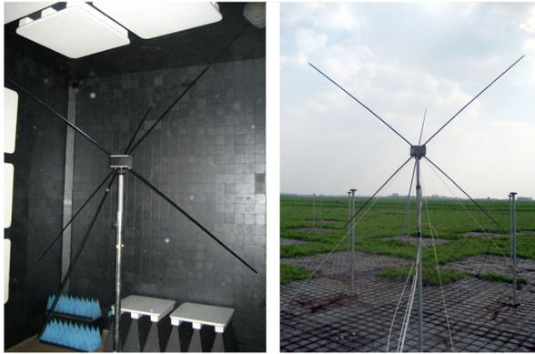
**Fig. 14** Tests with the prototype tripole antenna [13]. Left: Test setup in ASTRON chamber. Right: Setup in LOFAR station CS011 with 2 meters above the ground
