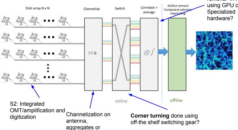
Correlation, RFI removal in real time using GPU cluster?
